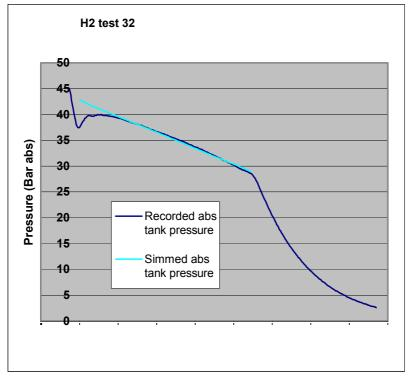
This cooling of the remaining liquid (and therefore any future gas to be vaporised from it's surface as the emptying progresses) means that the vapour-pressure (the tank pressure) will slowly drop over the burn time. In this graph, burnout was taken as the point when the liquid phase ran out (the graph suddenly steepens)
