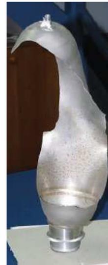
Another way to blow up the feed system is to let hot igniter gas back-flow through the injector. Don't let this happen.
