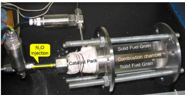
Figure 12. The restartable  $N_2O/PMMA$  hybrid rocket motor.
