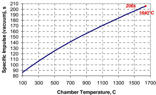
Figure 2. Theoretical specific impulse of nitrous oxide monopropellant thruster as a function of chamber temperature. (nozzle expansion ratio = 200)
