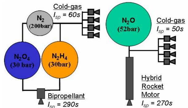
Figure 18. Schematics of Cold-Gas/Hybrid Rocket Motor propulsion system for a spacecraft.
