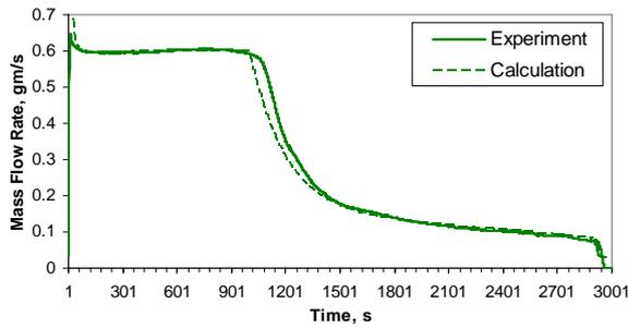
Figure 15. Results comparison for  $N_2O$  mass flow rate out of storage tank. (The initial mass flow rate curve step in the figure is because the flow out of tank was “controlled” by flow-meter heating the exhaust gas. When no liquid was left in the tank mass flow rate finally dropped to zero.)
