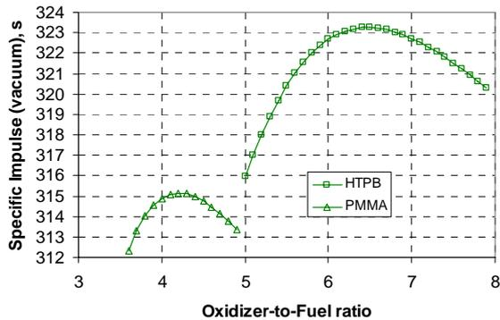
Figure 5. Theoretical specific impulse of nitrous oxide - solid fuel propellant combinations. (HTPB = hydroxyl-terminated polybutadiene; PMMA = polymethylmethacrylate)
