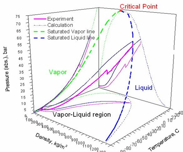
Figure 16. PDT-plot for nitrous oxide evaporation. (The initial pressure drop for experimental data is a dynamic pressure drop. The pressure spike for experimental data is due to heat of fusion passed to nitrous when the moisture condensed on the outside tank wall froze at  $0^\circ C$ .)
