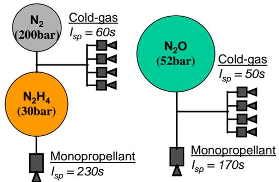
Figure 17. Schematics of Cold-Gas/Monopropellant propulsion system for a spacecraft.
