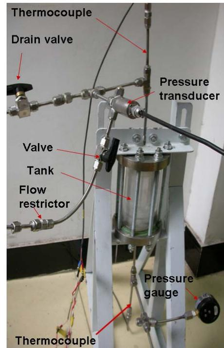
Figure 13. Experimental setup for liquefied gas testing.
