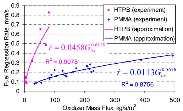
Figure 10. Solid fuel regression rates for N<sub>2</sub>O-fed hybrid rocket motor. ( $\dot{r}$  - fuel regression rate, mm/s;  $G_{ox}$  - oxidizer mass flux, kg/s/m<sup>2</sup>; R-squared value; The regression rates were obtained by weighing fuel grains before and after each firing.)
