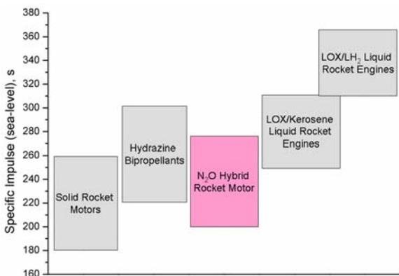
Figure 6. Performance comparison for selected booster propulsion. (LOX = liquid oxygen; LH<sub>2</sub> = liquid hydrogen; N<sub>2</sub>O = nitrous oxide. Data taken from sources [5,6])
