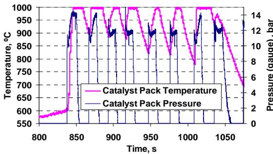
Figure 11. Restartable hybrid rocket motor test results. (Maximum temperature reading limit for K-type thermocouples was set to 1000°C)
