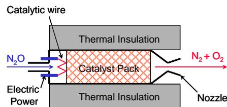
Figure 1. Nitrous oxide monopropellant thruster schematics.
