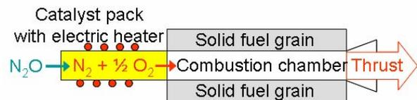
Figure 8. Schematics of N<sub>2</sub>O-fed hybrid rocket motor.
