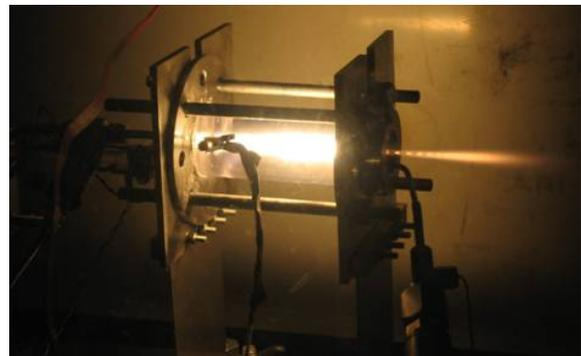
Figure 9. 4N-thrust N<sub>2</sub>O/PMMA hybrid rocket motor firing on thrust stand.
