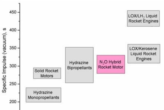
Figure 7. Performance comparison for selected upper-stage propulsion. (Data taken from sources [5,6])
