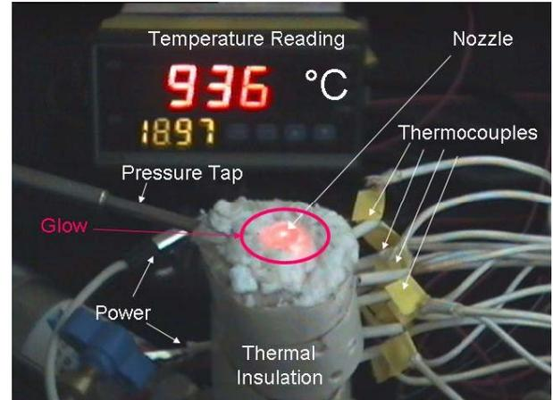
Figure 3. Nitrous oxide monopropellant firing. (The exhaust plume is invisible.)
