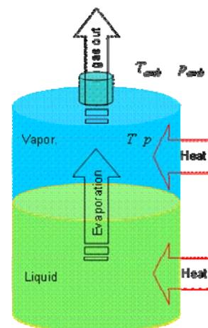
Figure 14. Sketch of storage tank self-pressurization by liquefied gas.
