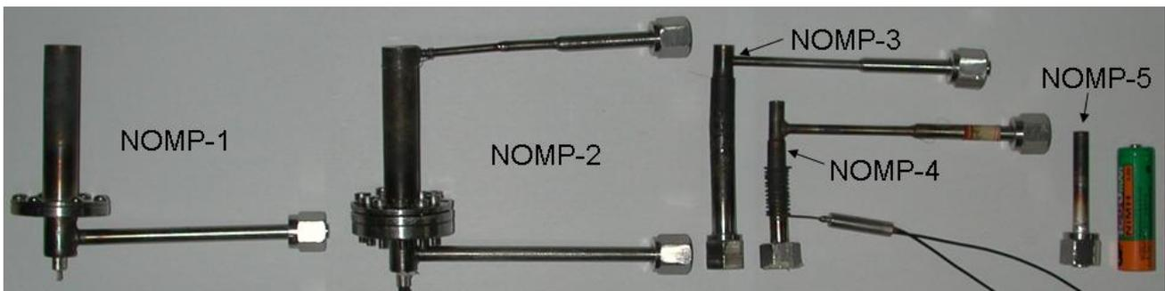
Figure 4. Nitrous Oxide Monopropellant Prototype (NOMP) designs.
