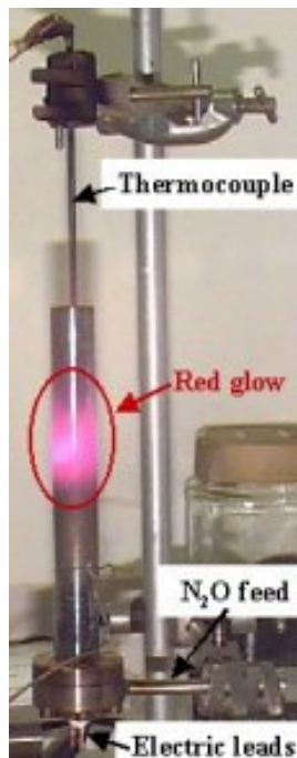
Fig. 2. Surrey-3 N 2 O monopropellant prototype design hot firing. (non-choked flow)
